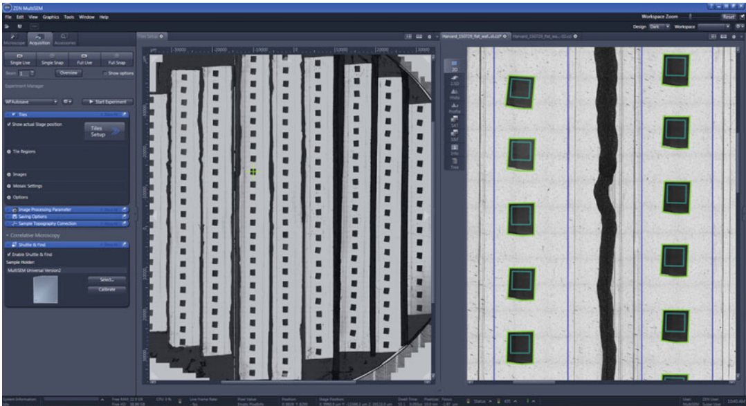
Fig. 4 Screenshot of ZEN for MultiSEM during experiment setup. A light microscopic overview image of a sample wafer with ultrathin sections cut with an ATUMtome and prepared as described before (left), regions of interest (in this case complete sections) labelled in green resulting from the automatic section detection (right) (Sample with courtesy of Jeff W. Lichtman, Harvard University)
