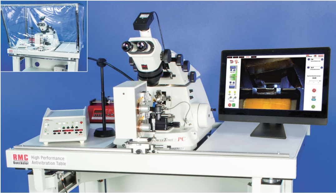
Fig. 1 Whole view of ATUMtome system. The ATUMtome is a combination of an ultramicrotome (PowerTome) and a tape collection device (ATUM), both operated by the same software. Antistatic device, water level control system, and air-activated antivibration microtomy table are included in the system. Inset shows the environmental chamber closed for more stable sectioning
