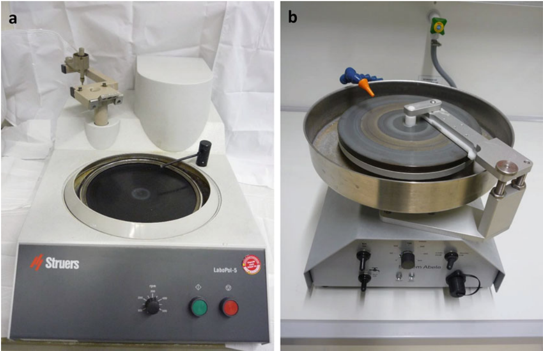
Fig. 4 Grinding and polishing devices: Different machines can be used to grind or polish the sample, two typical devices are depicted here. (a) The Labopol 5 (Struers) as it was used to prepare sample 2. (b) The mba (Abele GmbH) used for sample 1. Different grinding disks, abrasive papers, clay or suspensions containing diamond dust of specific grain sizes, or even clay can be used to ground the sample surface
